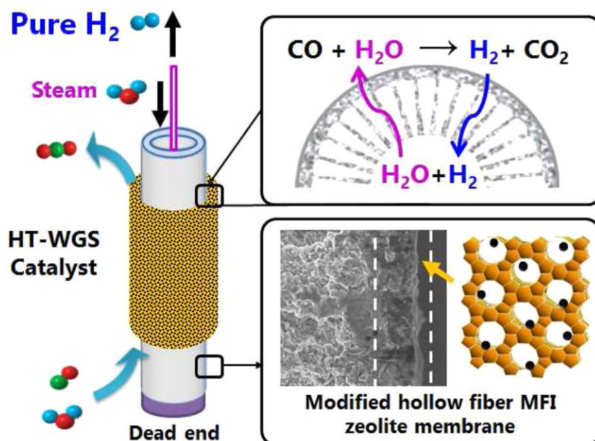
Figure 5. Schematic illustration of WGS membrane reactor with hollow fiber MFI zeolite membrane swept by steam.
